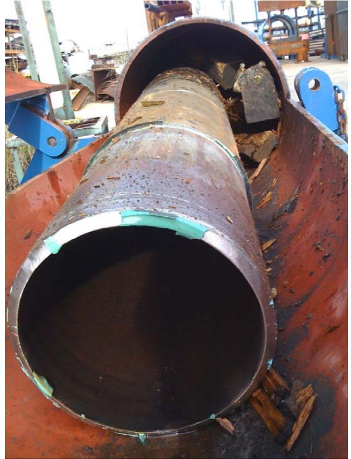
Figure 9: 12” Zap-Lok® Burst Test with Connection Separation.
